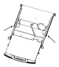
2. While one person positions the switch in the rack and holds it in place, the second person—using the screws provided with the rack mounting kit—loosely screws the front brackets to the rack.
